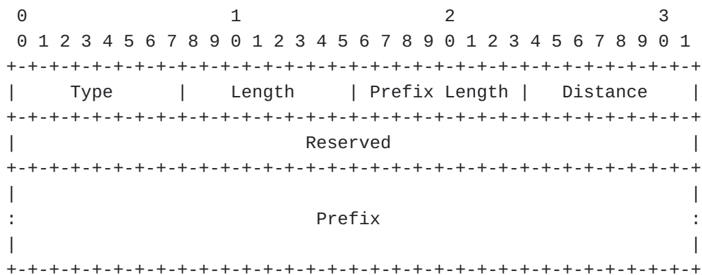
Figure 2: Vehicular Prefix Information (VPI) Option Format
