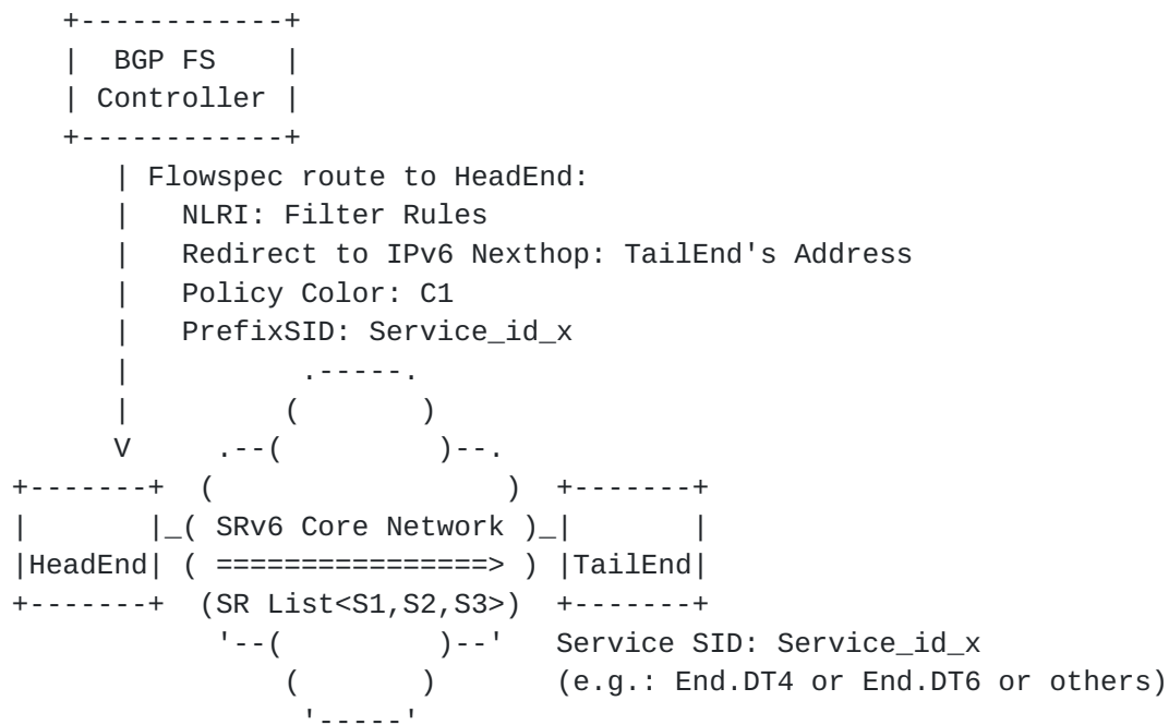
Figure 1: Steering the Flow into SRv6 Policy
