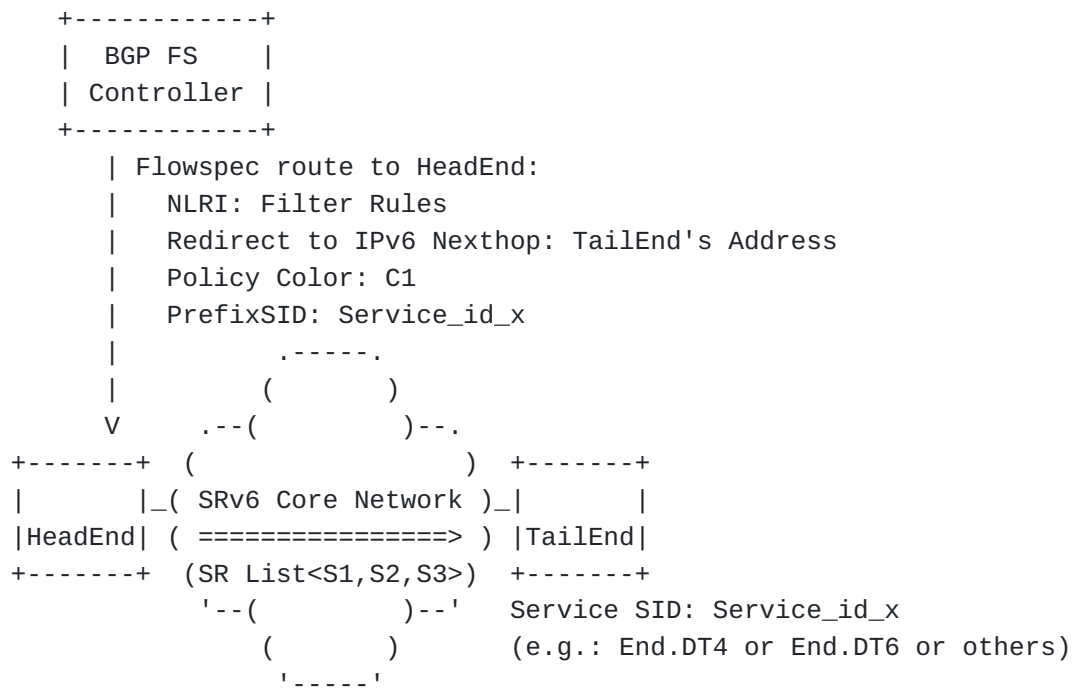
Figure 1: Steering the Flow into SRv6 Policy (Option 1)
