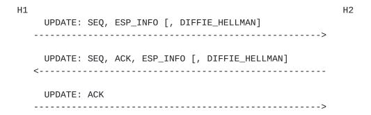
The host willing to update the ESP SA creates and sends an UPDATE message. The message contains the ESP\_INFO parameter containing the old SPI value that was used, the new SPI value to be used, and the index value for the keying material, giving the point from where the next keys will be drawn. If new keying material must be generated, the UPDATE message will also contain the DIFFIE\_HELLMAN parameter defined in [I-D.moskowitz-hip-rfc5201-bis].
