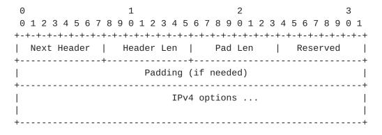
Next Header Identifies the data following this header Length in octets 8-bit unsigned integer. Length of the pseudo header in 8-octet units, not including the first 8 octets.
