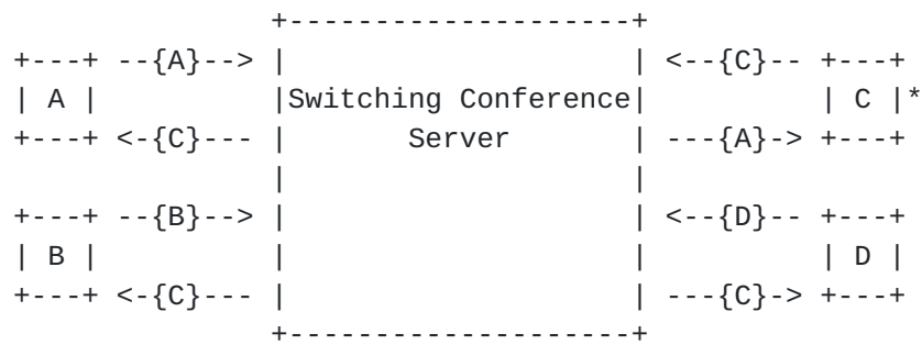
Figure 3 - Endpoint "C" is the Active Speaker
