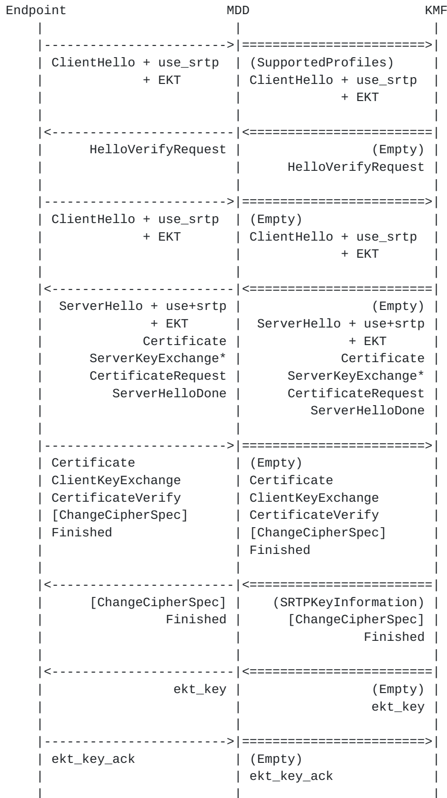
Figure 3: Sample DTLS-SRTP and EKT Exchange via a Tunnel
