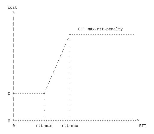
For RTTs below rtt-min, the link cost is just the nominal cost of a single hop, C. Between rtt-min and rtt-max, the cost increases linearly; abover rtt-max, the constant value max-rtt-penalty is added to the nominal cost.
