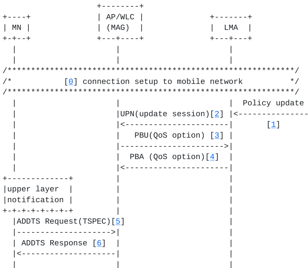
Figure 3: Network initiated QoS setup with WMM
