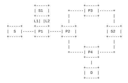
S=Source LSR, D=Destination LSR, S1,S2=service-nodes, L1,L2=links, P1,P2,P3,P4=Transit LSRs
