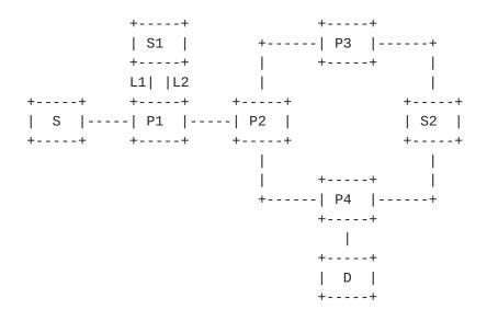
S=Source LSR, D=Destination LSR, S1,S2=service-LSRs, L1,L2=links, P1,P2,P3,P4=Transit LSRs
