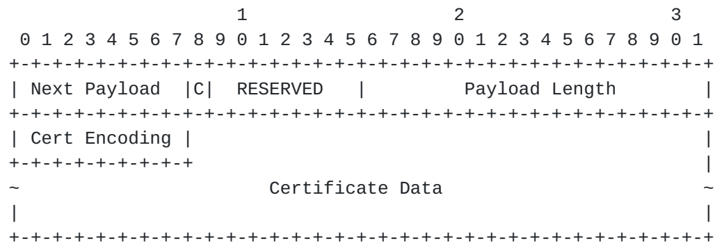
Figure 12: Certificate Payload Format
