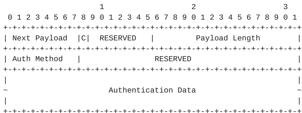
Figure 14: Authentication Payload Format
