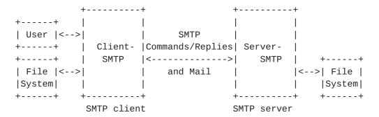
When an SMTP client has a message to transmit, it establishes a two-way transmission channel to an SMTP server. The responsibility of an SMTP client is to transfer mail messages to one or more SMTP servers, or report its failure to do so.
