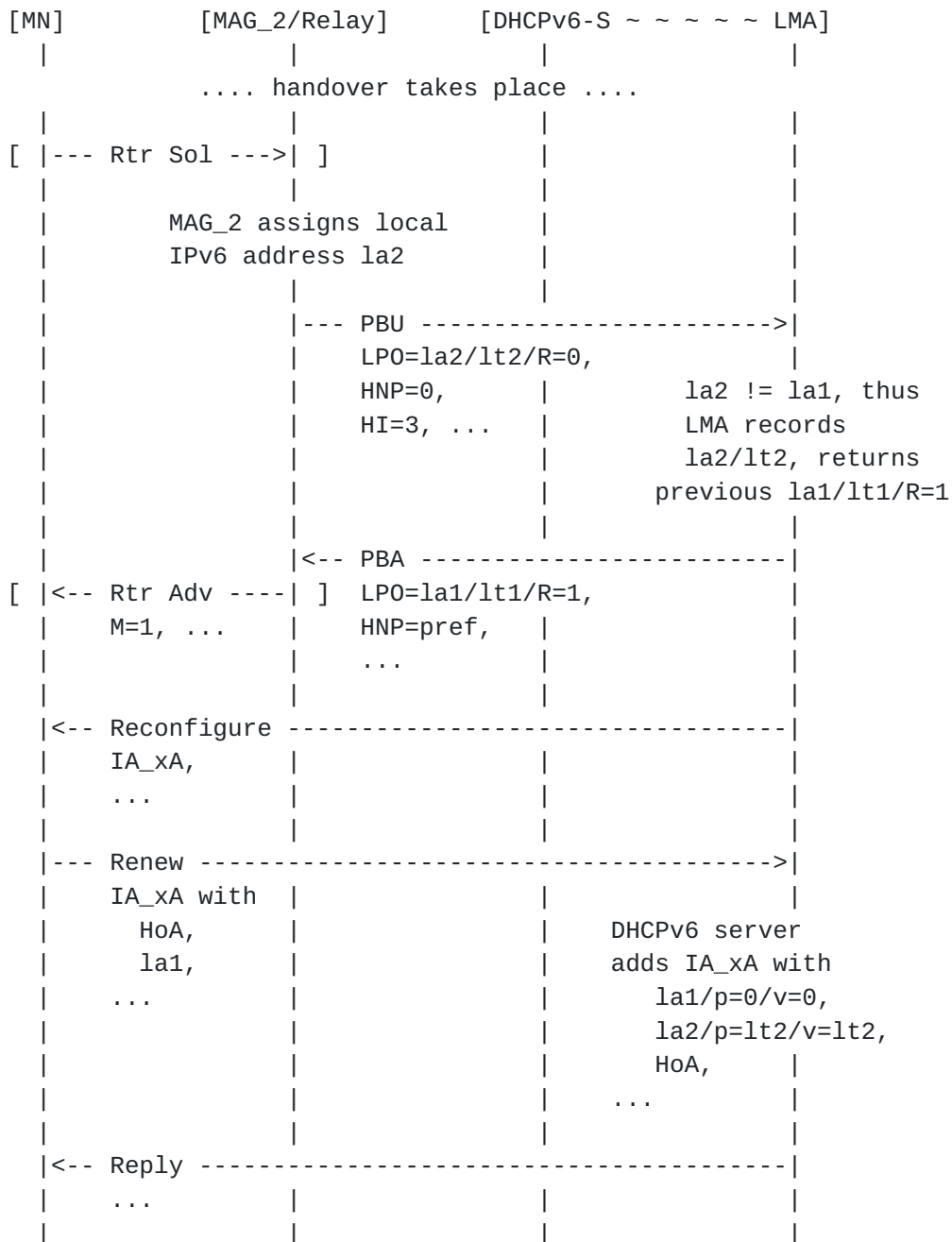
Figure 5: Local prefix change example using stateful DHCPv6 during a handover
