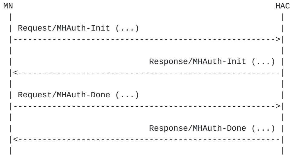
Figure 4: Authentication of the Mobile Node Using Shared Secrets
