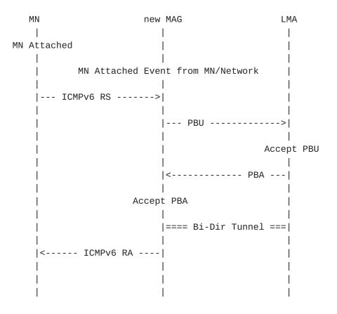
Figure 3: Mobile node's handover in PMIPv6
