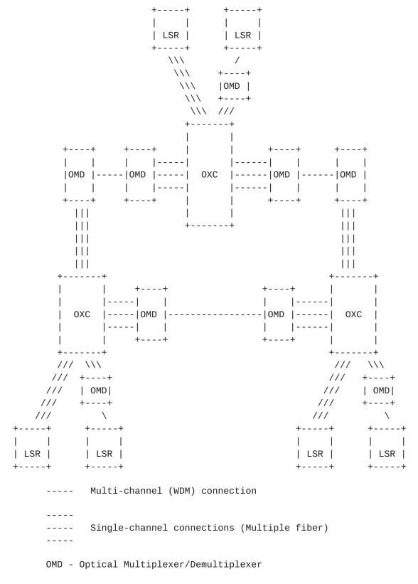
Fig. 1 - Optical IP Network with OXCs and Label Switch Routers
