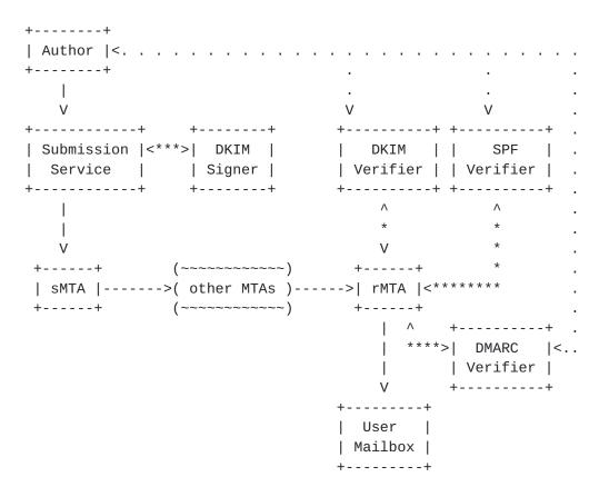
The above diagram shows the flow of messages through a DMARC-aware system. Solid lines denote the actual message flow; dotted lines involve Domain Name System queries used to retrieve message policy related to the supported message authentication schemes; asterisk lines indicate data exchange between message handling modules and message authentication modules.
