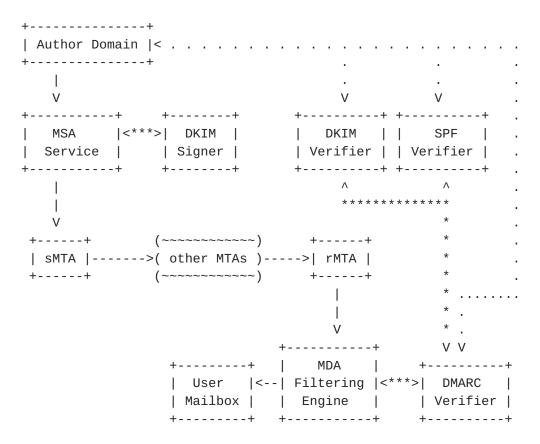
The above diagram shows a simple flow of messages through a DMARC-aware system. Solid lines denote the actual message flow, dotted lines involve Domain Name System queries used to retrieve message policy related to the supported message authentication schemes, and asterisk lines indicate data exchange between message handling modules and message authentication modules. "sMTA" is the sending MTA, and "rMTA" is the receiving MTA.
