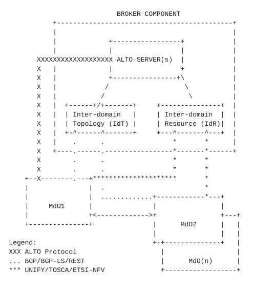
Figure 1: Broker-assisted Multi-operator Network Architecture
