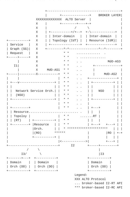
Figure 2: Broker-assisted 5GEx Info Exchange
