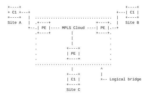
The set of PE devices interconnected via MPLS appears as a single 802.1d bridge/switch to customer C1. Each PE device will learn remote MAC addresses on LSPs (and keeps learning directly attached MAC addresses on customer facing ports).
