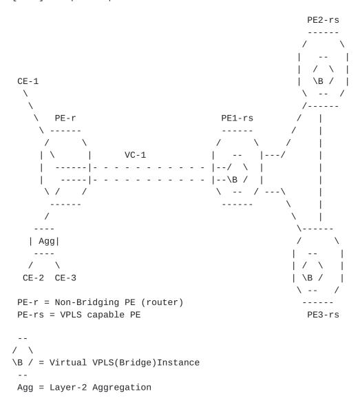
As shown in this figure, the PE-r device creates a point-to-point tunnel LSP to a PE-rs device. Then for every access port that needs to participate in a VPLS service, the PE-r device creates a point-to-point [MARTINI-ENCAP] VC that terminates on the physical port at the PE-r and terminates on the virtual bridge instance of the VPLS
