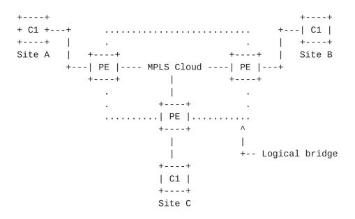
The set of PE devices interconnected via transport tunnels appears as a single 802.1D bridge/switch to customer C1. Each PE device will learn remote MAC addresses to VC LSP associations and learns directly attached MAC addresses on customer facing ports.
