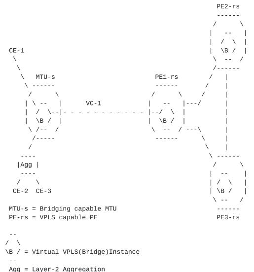
The MTU-s device and the PE-rs device treat each spoke connection like an access port of the VPLS service. On access ports, the
