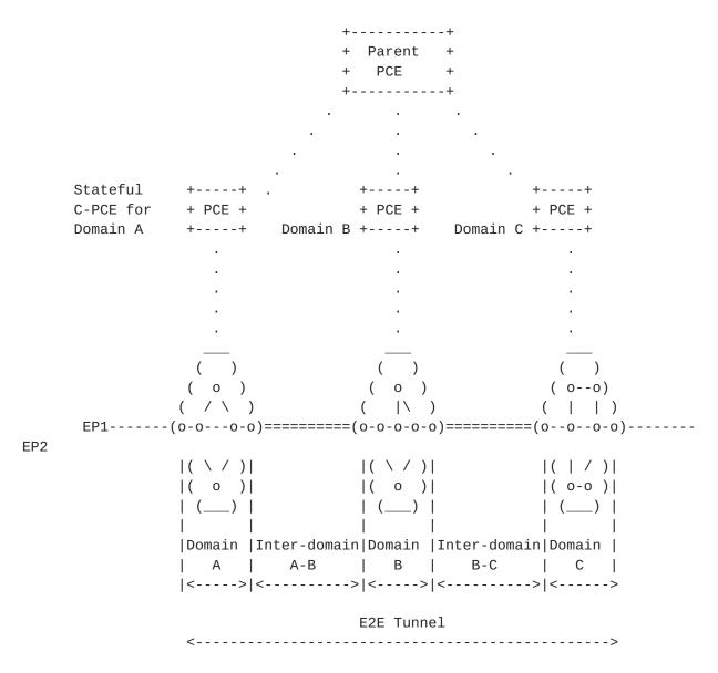
Figure 1: Multi-domain LSP stitching for an end-to-end tunnel
