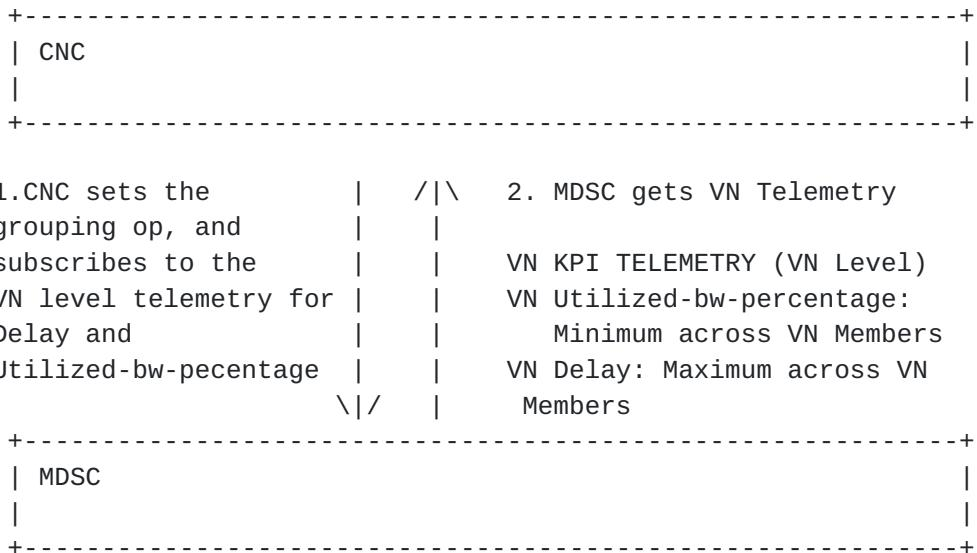
The ACTN VN TE-Telemetry Model augments the basic ACTN VN model to enhance VN monitoring capability. This monitoring capability will facilitate proactive re-optimization and reconfiguration of VNs based on the performance monitoring data collected via the ACTN VN Telemetry YANG model.
