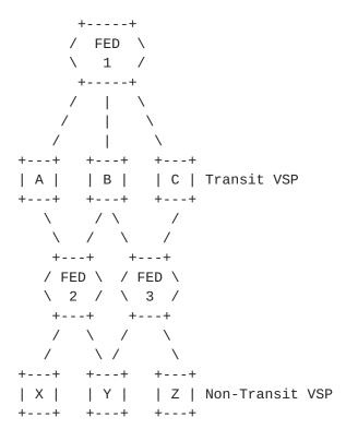
X, Y, and Z are terminating VSPs which serve as SIP providers for end-customers. A, B, and C are VSPs offering transit into a federation to members of other federations.
