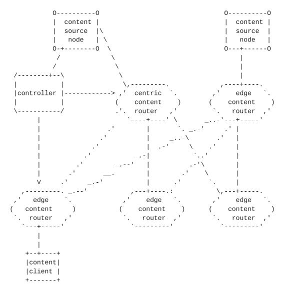
The figure below depicts the roll of a centralized controller in the ICN. Content routing tables of the routers and caching policy of the centric content router (CCR) are all generated by the controller according to its analysis of collected information, and ISP policies can be enforced. When a content router starts up, it discovers the
