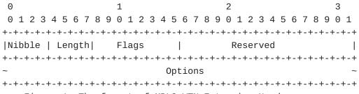
Figure 1. The format of MPLS VTN Extension Header
