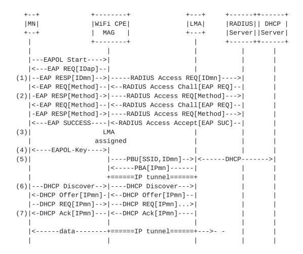
Figure 2: PMIPv6 inter-working with WPA2-802.1X access authentication against a RADIUS server
