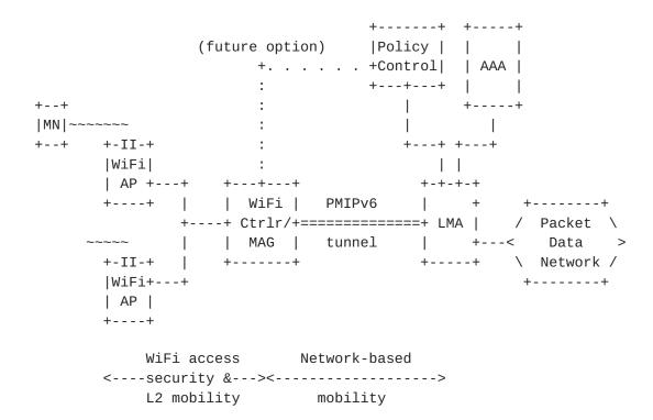
Figure 1: Integration of the WiFi radio technology to provide trusted access to mobile operator networks
