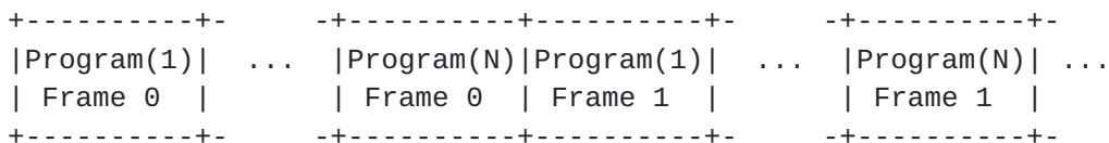
Figure 2. Interleaving of multiple programs in an E-AC-3 bit stream
