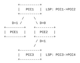
With this new PCEP session topology, we first configure PCC1->PCC2, PCE1 computes the shortest path as it is the only LSP in the disjoint-group that it is aware of: R1->R3->R4->R2->PCC2 (shortest path). When PCC3->PCC4 is configured, PCE2 must compute a disjoint path for this LSP. The only solution found is to move PCC1->PCC2 LSP on another path, but PCE2 cannot do it as it does not have delegation for this LSP. In this setup, PCEs are not able to find a disjoint path.
