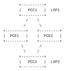
In the figure above, we consider a loadbalanced PCE architecture, so PCE1 is responsible to compute paths for PCC1 and PCE2 is responsible to compute paths for PCC2. When PCE1 triggers an LSP update for LSP1, it sends a PCUpdate message to PCC1 for LSP1 containing the new parameters. PCC1 will take the parameters into account and will send a PCReport to PCE1 and PCE2 reflecting the changes. PCE2 will so be notified of the change only after receiving the PCReport from PCC1.
