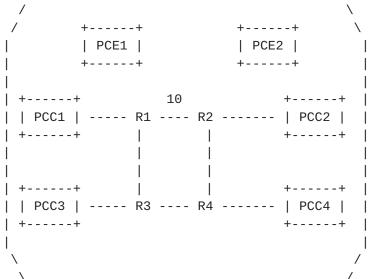
In the figure above, we want to create two link-disjoint LSPs: PCC1->PCC2 and PCC3->PCC4. In the topology, all link metrics are equal to 1 except the link R1-R2 which has a metric of 10. The PCEs are responsible for the path computation and PCE1 is the active PCE for all PCCs in the nominal case.
