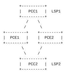
In the figure above, we consider a loadbalanced PCE architecture, so PCE1 is responsible to compute paths for PCC1 and PCE2 is responsible to compute paths for PCC2. When PCE1 triggers an LSP update for LSP1, it sends a PCUpd message to PCC1 for LSP1 containing the new parameters. PCC1 will take the parameters into account and will send a PCRpt message to PCE1 and PCE2 reflecting the changes. PCE2 will so be notified of the change only after receiving the PCRpt message from PCC1.
