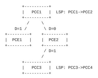
With this new PCEP session topology, we first configure PCC1->PCC2, PCE1 computes the shortest path as it is the only LSP in the disjoint association group that it is aware of: R1->R3->R4->R2->PCC2 (shortest path). When PCC3->PCC4 is configured, PCE2 must compute a disjoint path for this LSP. The only solution found is to move PCC1->PCC2 LSP on another path, but PCE2 cannot do it as it does not have delegation for this LSP. In this setup, PCEs are not able to find a disjoint path.
