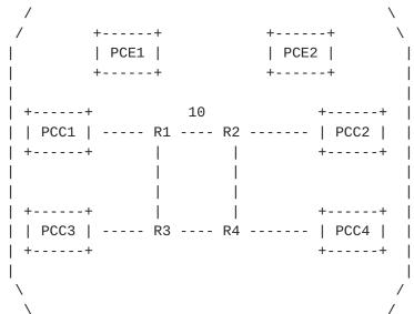
In the figure above, the requirement is to create two link-disjoint LSPs: PCC1->PCC2 and PCC3->PCC4. In the topology, all links cost metric is set to 1 except for the link 'R1-R2' which has a metric of 10. The PCEs are responsible for the path computation and PCE1 is the active primary PCE for all PCCs in the nominal case.
