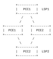
In the figure above, we consider a load-balanced PCE architecture, so PCE1 is responsible to compute paths for PCC1 and PCE2 is responsible to compute paths for PCC2. When PCE1 triggers an LSP update for LSP1, it sends a PCUpd message to PCC1 containing the new parameters for LSP1. PCC1 will take the parameters into account and will send a PCRpt message to PCE1 and PCE2 reflecting the changes. PCE2 will so
