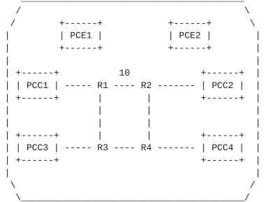
In the figure above, the requirement is to create two link-disjoint LSPs: PCC1->PCC2 and PCC3->PCC4. In the topology, all links cost metric is set to 1 except for the link 'R1-R2' which has a metric of 10. The PCEs are responsible for the path computation and PCE1 is the active primary PCE for all PCCs in the nominal case.
