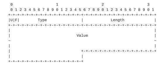
The TLV format definition in <a href="[RFC5036">[RFC5036]</a> Section 3.3 can be used for the Explicit Path TLV carrying the specified path of the Segment List.
