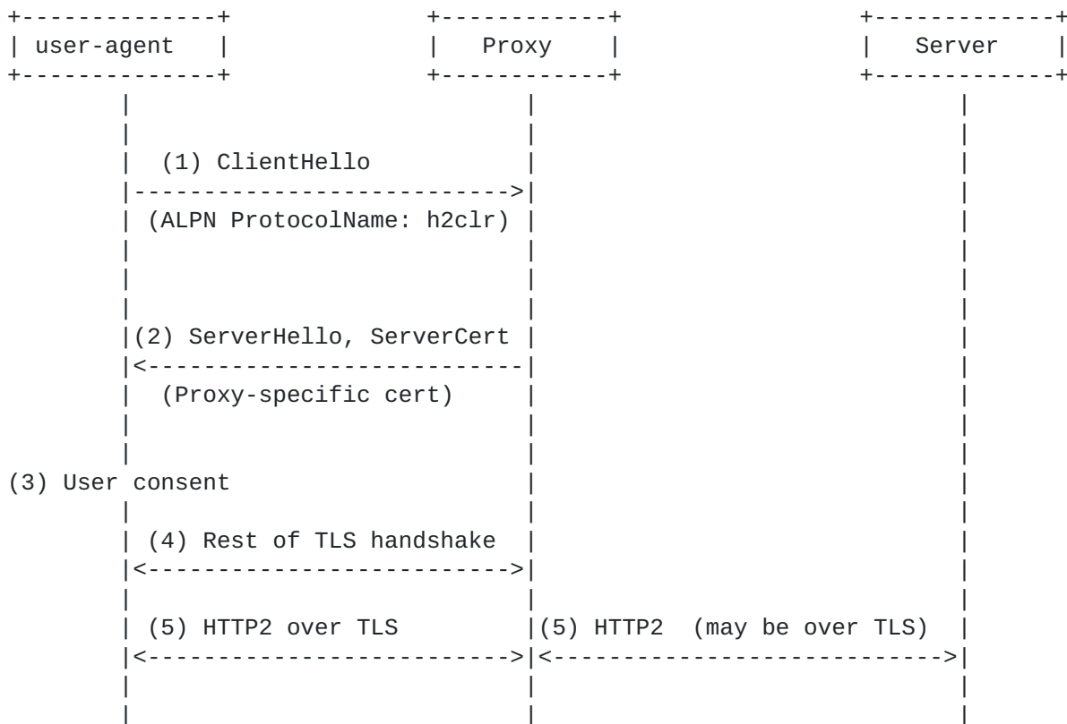
Figure 2: TLS Handshake with Proxy certificate
