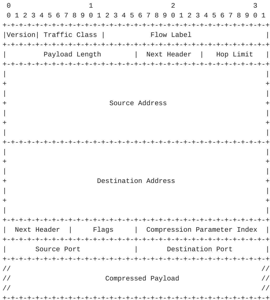
Figure 1: Packet format when using Four-bytes Exclusion Extension
