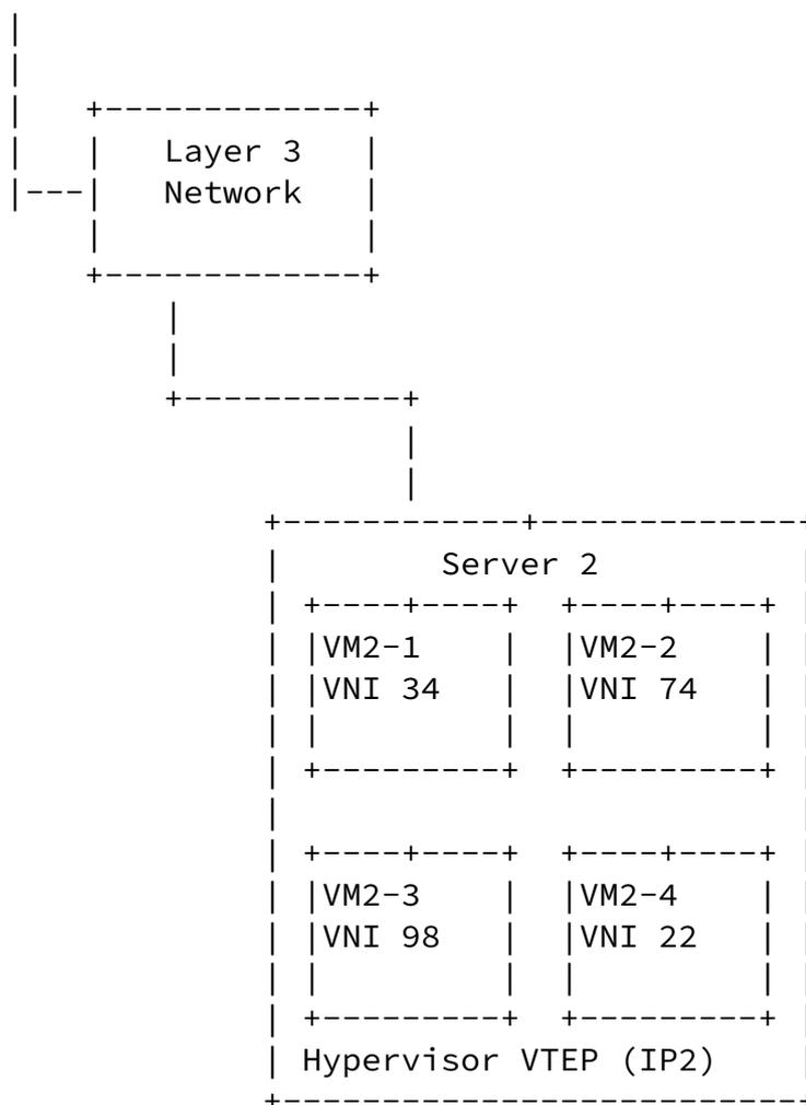
Figure 3 VXLAN Deployment - VTEPs across a Layer 3 Network
