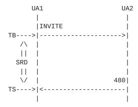
The following flow provides an example of identifiable events necessary for inputs in calculating SRD during a failed session setup attempt with a redirect (e.g. 302 Moved Temporarily):
