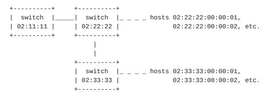
Since these two identifiers when concatenated must form a unicast LAA, the settings of two bits in the first byte of the switch identifier are fixed: the least significant bit must be 0 to indicate a unicast address, and the second-least significant bit must be 1 to indicate a LAA. To cater for variable length switch identifiers, some means of
