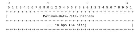
The Maximum-Data-Rate-Upstream AVP contains an 8-octet unsigned integer, indicating the numeric value of the subscriber's Access Line maximum upstream data rate. The rate is coded in bits per second.
