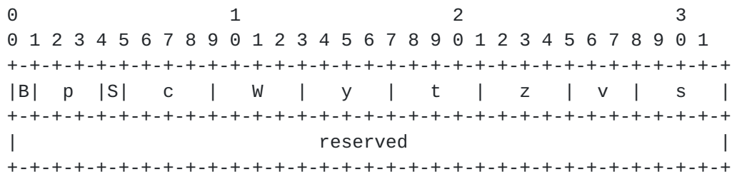
Figure 4: G.689.1 Application Code Encoding
