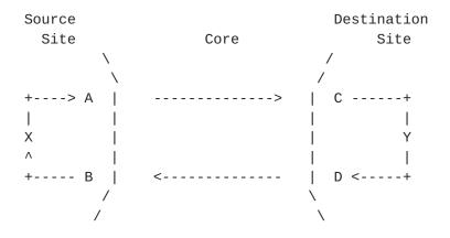
Figure 1: Square Routing Packet Flow
