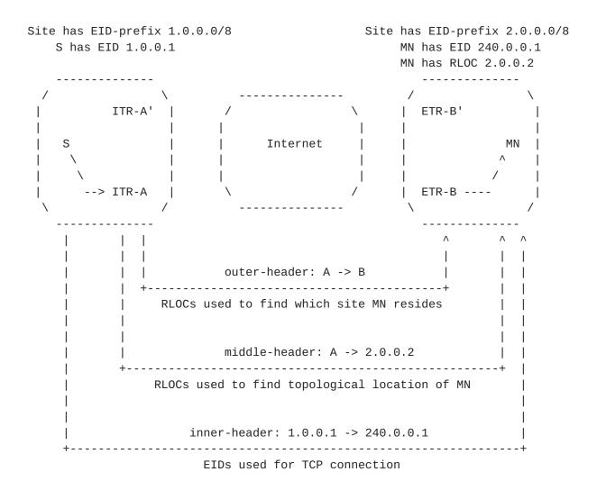
Figure 2: Mobile Node Roaming into a LISP Site
