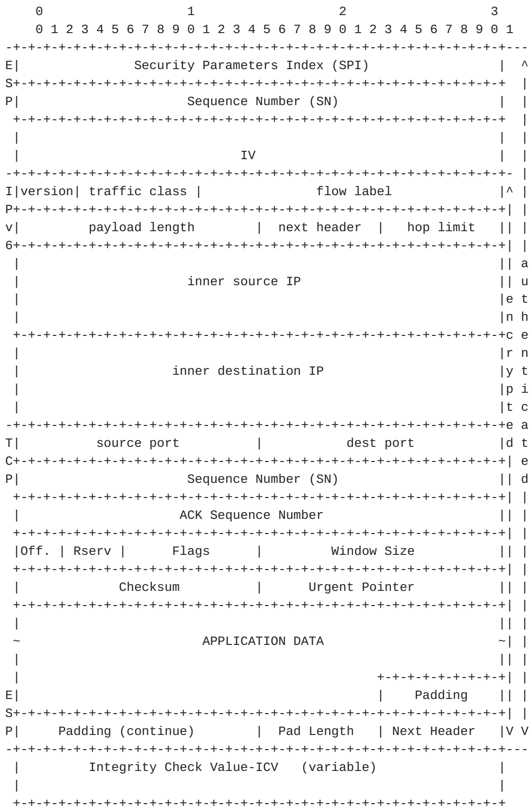
Figure 5: Standard IoT Single TCP Session VPN Packet Description
