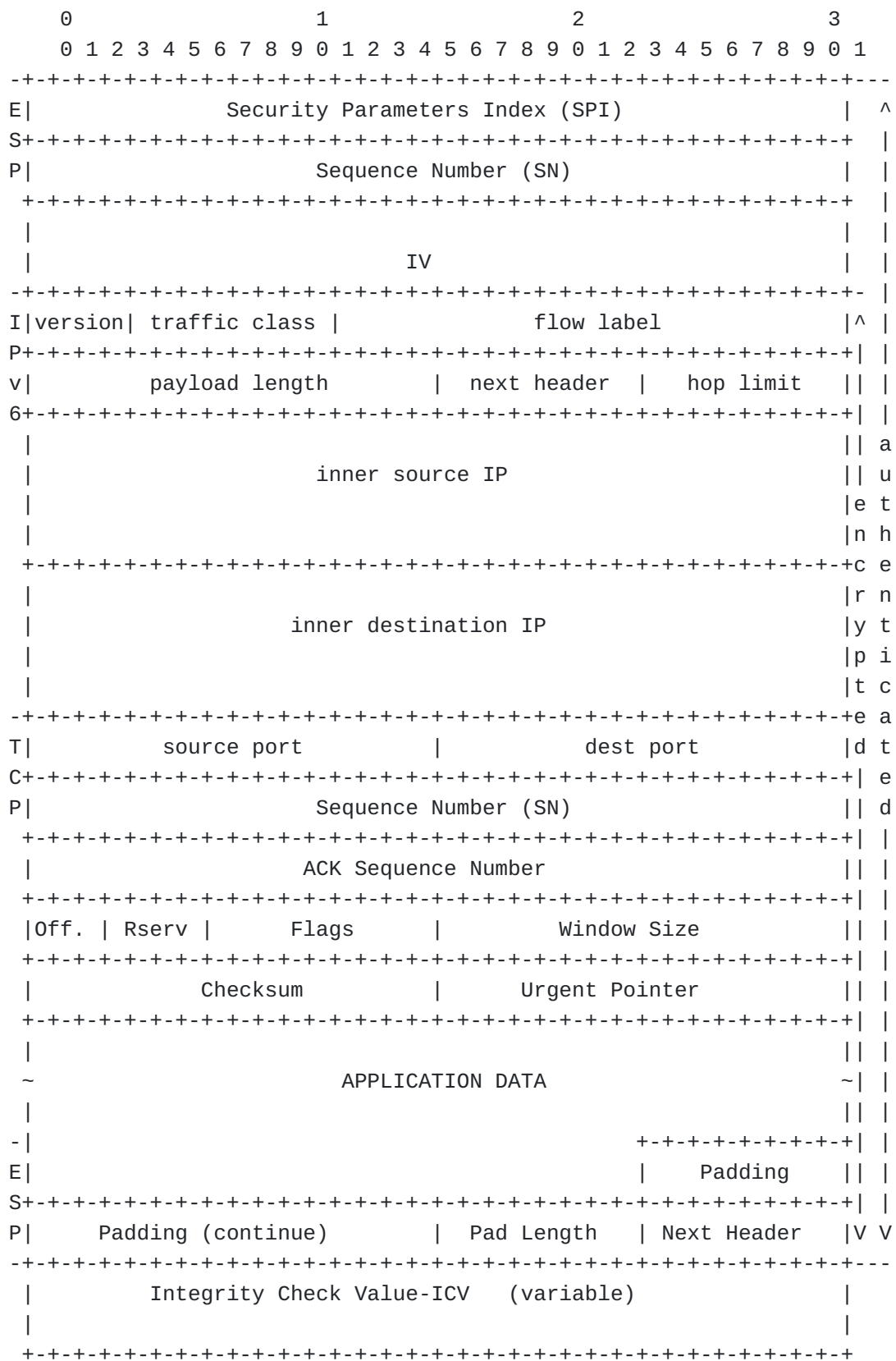
Figure 7: Standard ESP VPN Packet Description
