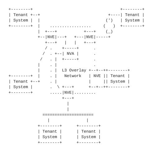
Figure 1: Generic Reference Model for Network Virtualization Overlays [<u>RFC7365</u>]
