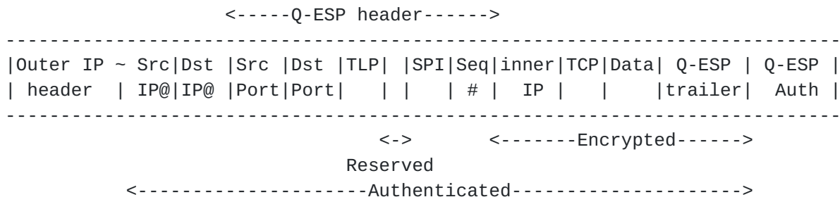
Figure 3: Q-ESP in tunnel mode
