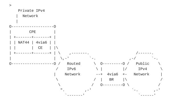
4via6 CE has two functionalities. The first is to generate an IPv4 address or an shared IPv4 address and port-set. The second is to translate an IPv4 packet from/to an IPv6 packet across IPv6 network. When an unique IPv6 prefix is assigned to each CPE from SP's network, 4via6 CE in the CPE generates IPv4 address or shared IPv4 address and port-set with 4rd address mapping rule defined in <u>[I-D.murakami-</u> softwire-4rd].
