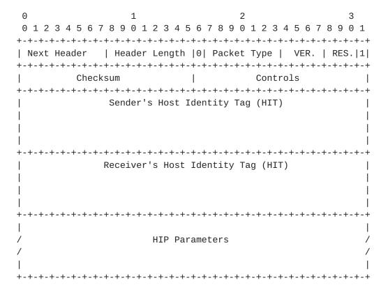
The HIP header is logically an IPv6 extension header. The HIP protocol specification [RFC5201] defines handling only for Next Header value decimal 59, IPPROTO\_NONE, the IPv6 'no next header' value. This document describes processing for Next Header values other than decimal 59 which indicates that there is either more extensions header or data following the HIP header.
