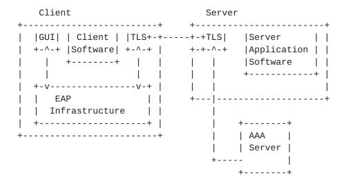
The above diagram shows the typical deployment. The client has software that either includes a UI for some EAP methods, or else is able to invoke some operating system EAP infrastructure that takes care of the user interaction. The server is configured with the address and protocol of the AAA server. Typically the AAA server communicates using the RADIUS protocol with EAP ([RADIUS] and [RAD-EAP]), or the Diameter protocol ([Diameter] and [Dia-EAP]).
