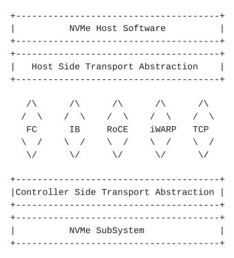
This document describes the application scenarios and capability requirements of the Ethernet-based NVMe that implements automatic device discovery, domain management, and fault notification similar to FC.
