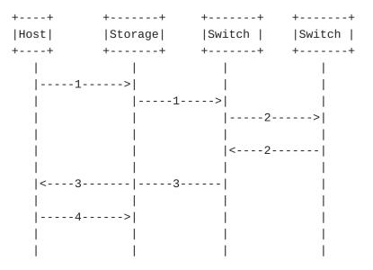
Fault detection: The host can detect the fault status of the storage device and quickly switch to the standby path.
